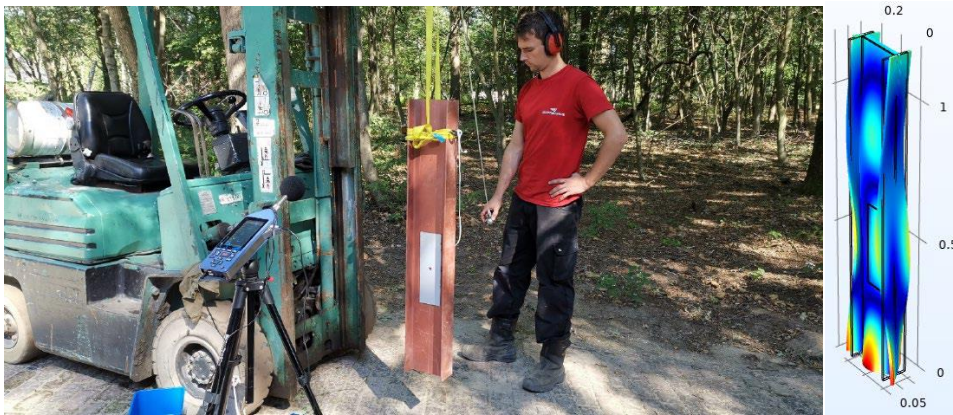
Figure 8: Setup of the small-scale validation on the left and the modelled beam on the right
