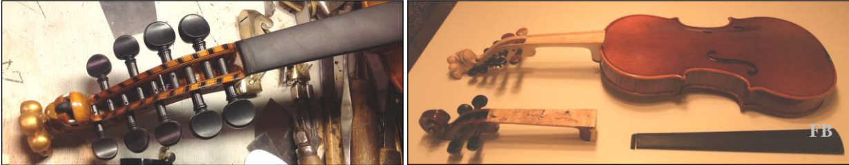
Figure 9: A HF pegbox and neck. Right: The Guarneri model violin fitted with a HF neck. The violin fingerboard (FB) was carved flatter and hollowed out for the sympathetic strings on the HF. Response curves were measured for each step in the working process.
