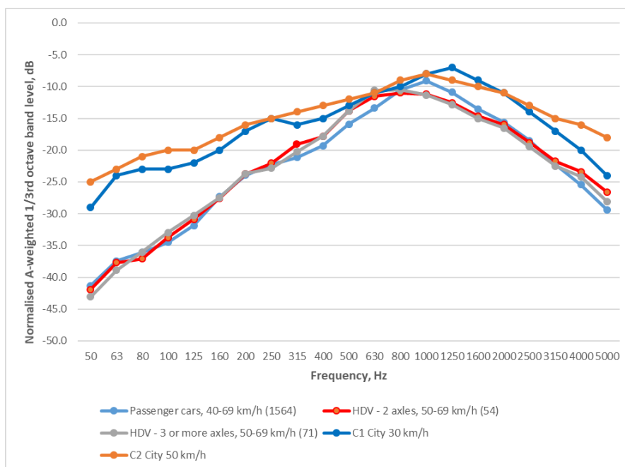
Figure 5: Normalised A-weighted 1/3 rd octave band spectra for passenger cars and heavy-duty vehicles, measured by SINTEF in 2015 [4,5]. Number of vehicles in parenthesis
