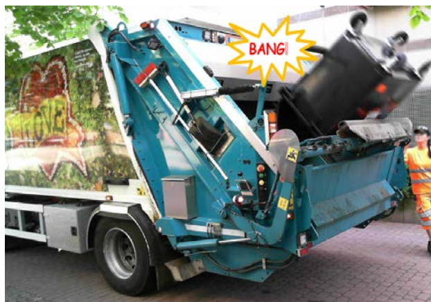
Figure 5. Impact noise is created when the waste container hits against the limiter bar.
